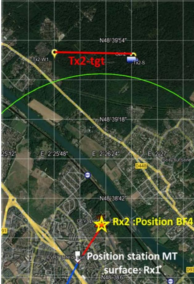
Figure 10.6 Positioning map of the source dipole in Sénart Forest (TX2 or TX), the borehole probe at the bottom (RX2), and the surface MT station (RX1).
