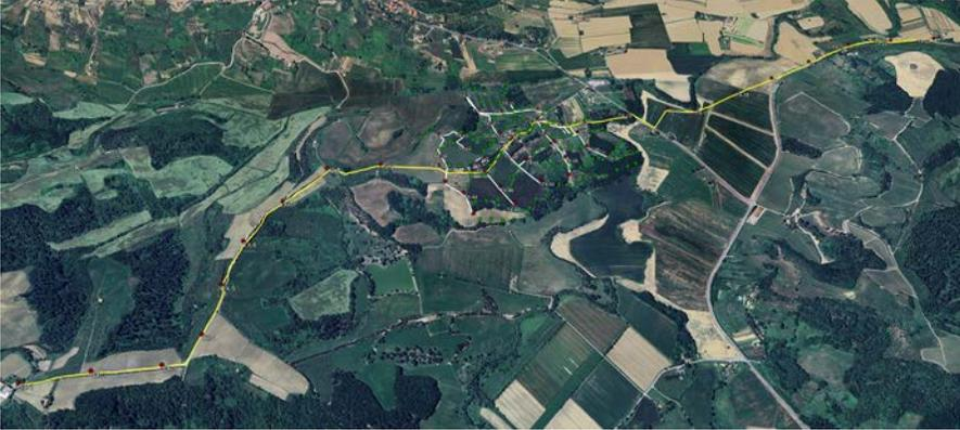
Figure 5.5 Aerial view of transmissions points (in red) and receivers points (in green). The longest distance on injection dipole along the main axis (in yellow, between TX1 and TX 23) is about 5.5 km. The white lines, more central on the figure, show the cables used for shorter distance transmissions, inside the area of interest.
