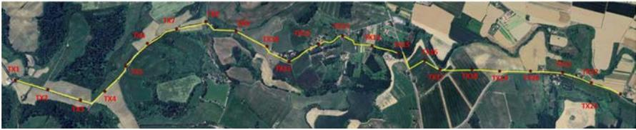
**Figure 5.7** Location of the transmission's electrodes on main central axe. Pole A was in TX1 and pole B was moving on all TX from TX2 to TX23. A backward acquisition was done on the main axe, with pole A fixed at TX23 and pole B moving backward on TX21, TX19, TX17, ..., TX1 (one out of two).
