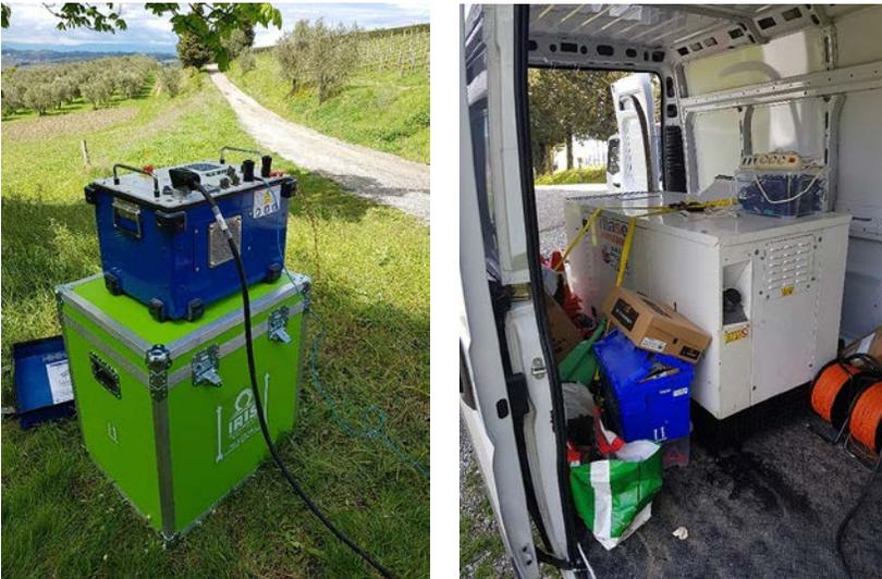
**Figure 5.2** On the left, high power transmitter of 6 kW. On the right, the three-phase 15 kVA motor generator which powers the transmitter.
