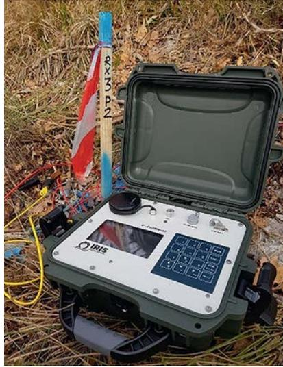
Figure 5.4 Receiver box deployed at the wooden stick location.
