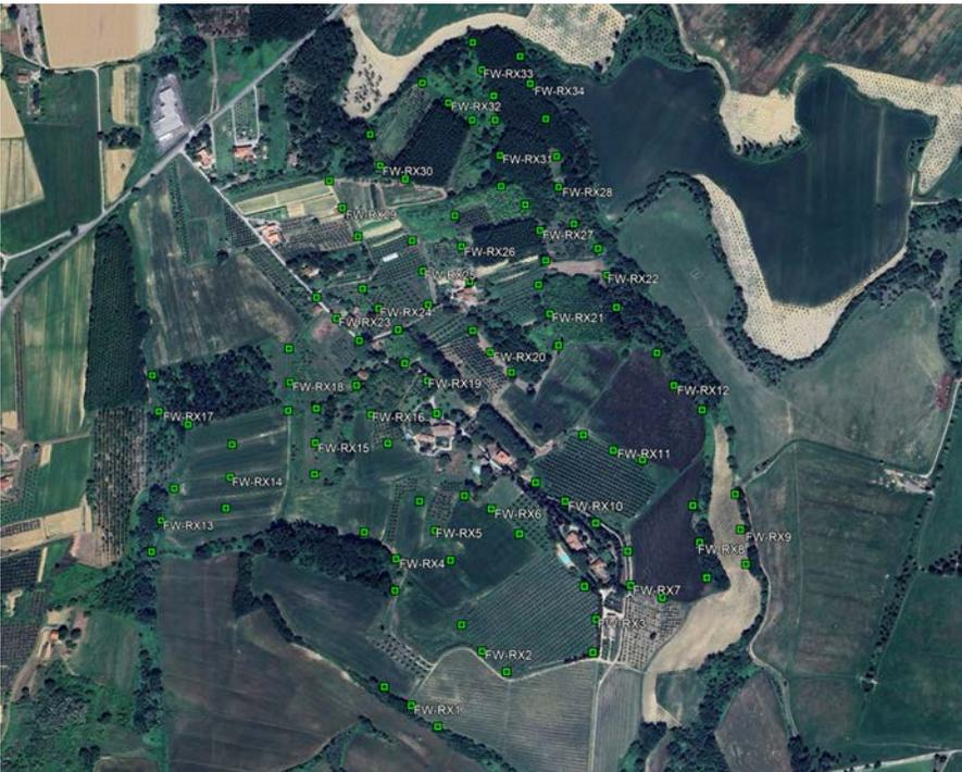
Figure 5.6 Layout of 102 electrodes and 34 recording units in the area of interest.
