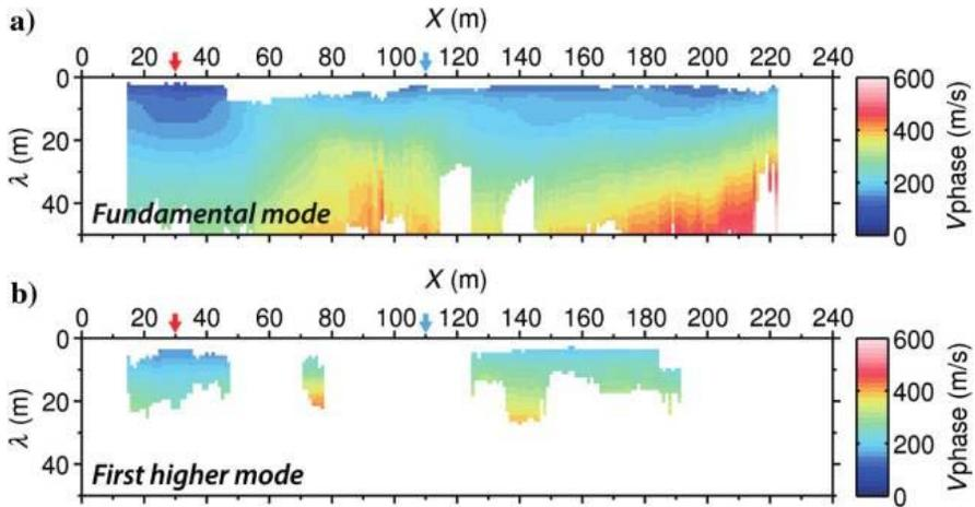
Figure 6.10 Pseudo-sections of SW phase velocity picked for (a) the fundamental and (b) first higher modes along the line after dispersion stacking, represented as a function of the wavelength  $\lambda$  and the spread mid-point position. From Pasquet and Bodet (2017).
