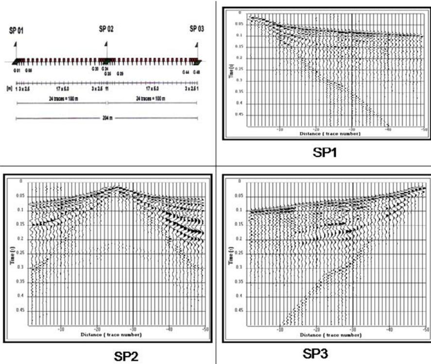
Figure 6.2 Refraction seismic acquisition: spread and the three-common shot-gathers of the 10EST04 profile. Adapted from Mendes et al. (2014).
