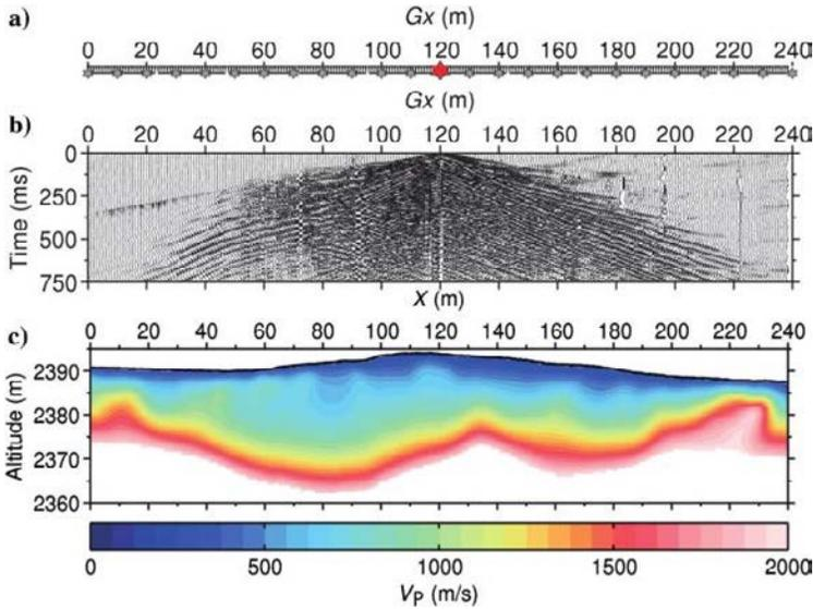
**Figure 6.6** (a) Layout of the seismic acquisition setup, with 240 geophones (gray triangles) spaced every 1 m and 25 shots (gray stars) spaced every 10 m. (b) Example of a shot gather for a source located at 120 m (red star in a). (c) Final P-wave velocity model obtained from P-wave travel time tomography. The topography extracted from airborne LiDAR data is represented with a solid black line. From Pasquet and Bodet (2017).
