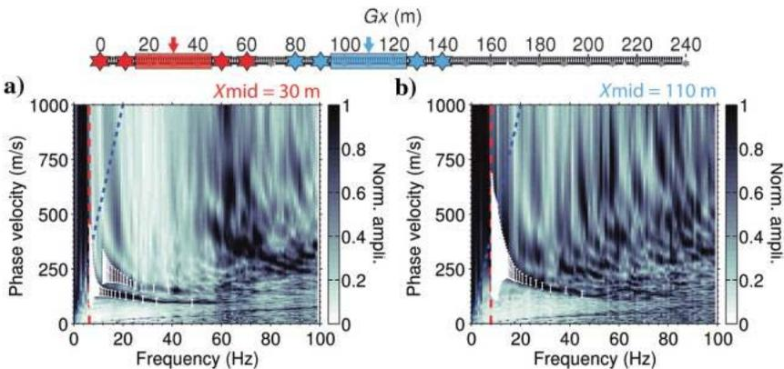
Figure 6.9 Stacked dispersion images extracted at (a)  $X_{mid} = 30$  m and (b)  $X_{mid} = 110$  m with picked dispersion curves (white error bars) of the fundamental (0) and first higher (1) modes. The uncertainty range is defined according to the workflow described in O'Neill (2003). Dispersion curves are limited to a frequency defined with a spectral amplitude threshold of 2.5% (dashed red line), or up to a wavelength of 50 m (dashed blue line). From Pasquet and Bodet (2017).
