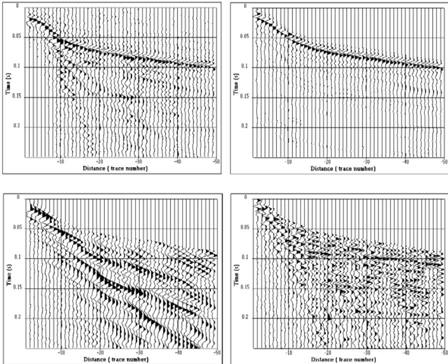
**Figure 6.4** Deconvolution and wave separation for shot point 1 of the 10EST04 profile. Top left: deconvolution by spectrum equalization in the 12–160 Hz frequency bandwidth. Top right: Extraction of direct and refracted waves by SVD filter. Bottom left: Extraction of surface waves (Pseudo Rayleigh waves) by F-K filter. Bottom right: Reflected waves and residual noise. Adapted from Mendes et al. (2014).
