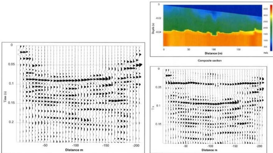
**Figure 6.5** Reflectivity section for 10EST04 profile: Left: Single fold section derived from reflection processing of off-end shots. Bottom right: Upward continuation of single-fold section using reflectivity derived from tomographic velocity model. Top right: Time converted velocity model obtained by tomographic inversion. Adapted from Mendes et al. (2014).
