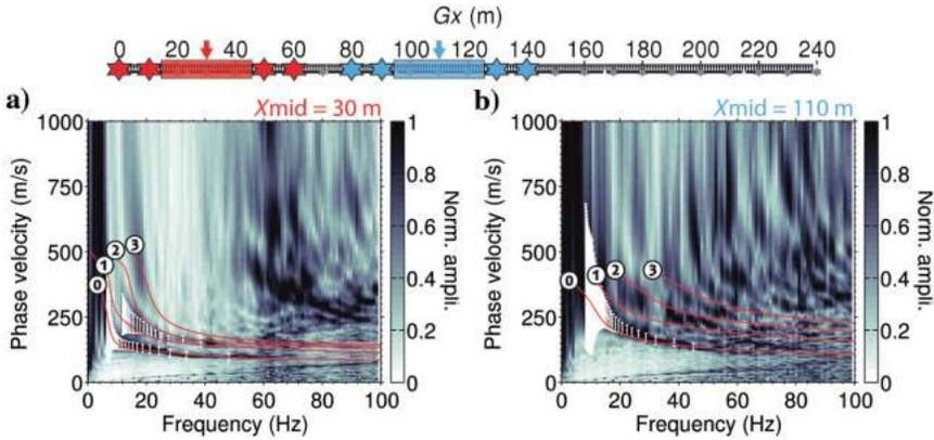
Figure 6.12 Stacked dispersion images extracted at (a)  $X_{mid} = 30\text{ m}$  and (b)  $X_{mid} = 110\text{ m}$  with picked (white error bars) and calculated (solid red lines) dispersion curves represented for the fundamental (0), the first (1), second (2), and third (3) higher modes. From Pasquet and Bodet (2017).
