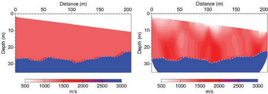
**Figure 6.3** *Tomographic inversion for the 10EST04 profile. Left: Input model  $V1 = 1,300$  m/s and  $V2 = 3,250$  m/s provided by the Plus-Minus method. Right: Velocity model generated by tomographic inversion. The result exhibits velocity with strong lateral variations for the heterogeneous shaly mudstone over a bedrock of compact limestone. Adapted from Mendes et al. (2014).*
