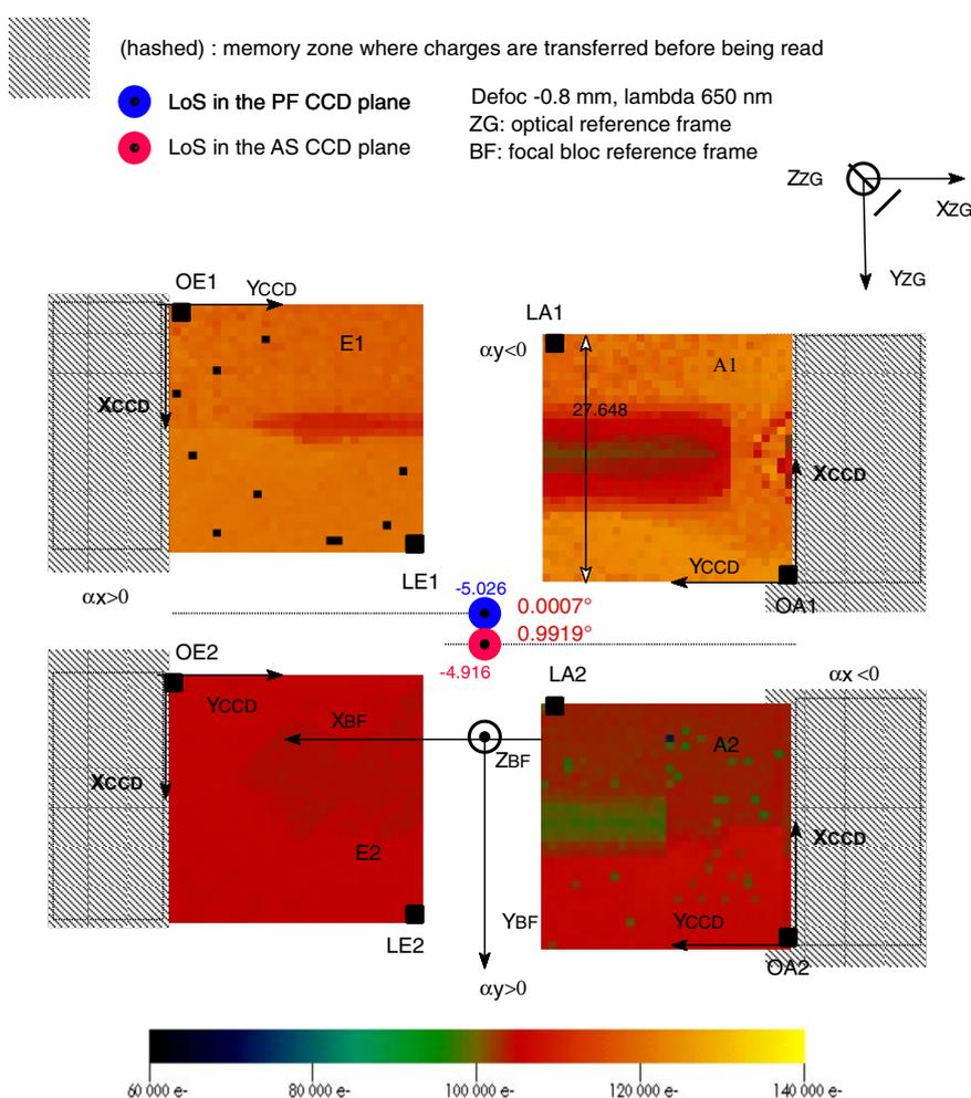
For each CCD,  $O_{CCD}$  is the origin of the CCD;  $L_{CCD}$  is located opposite to the origin.
