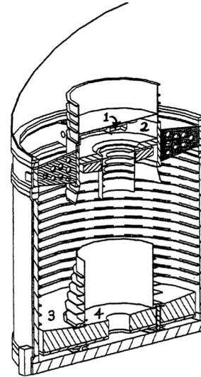
**Fig. I.2.3.** An exploded view of the payload of STARS. © ESA. The numbers refer to: 1) location of the photometric detector; 2) location of the second instrument: Lyman Alpha Monitor (LAM); 3) Outer section of the main mirror; 4) inner section of the main mirror.
