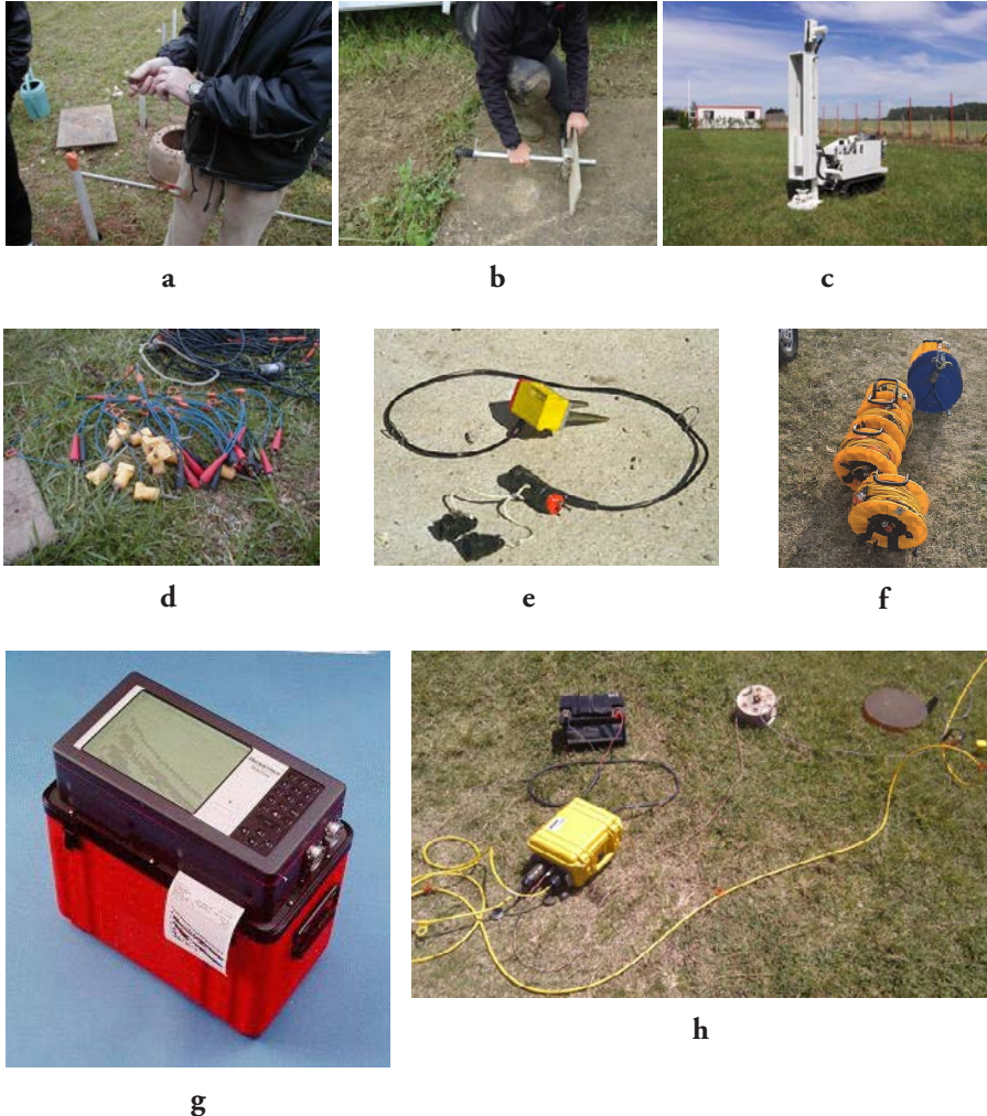
Figure 2.6 Field equipment. Source: explosive, gun, weight drop (a, b, c: Apec document); sensors: vertical and horizontal geophones (d, e: IFPEN document), cables (f: IFPEN document); recorders: Geometrics Strataview (g: IFPEN document), Geometrics geode (h: GEO2X document).
