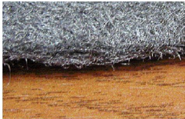
Metal fabric thickness 2-6 mm, Fiber diameter - 40\text{mkm} , Heat resistance - up to 600^\circ\text{C}
