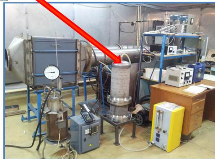
Experimental research of gas filter at test facility CIAΦ-1 (test facility for aerosol filter testing)
