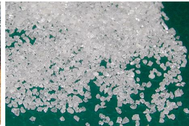
Fused corundum (screened size \text{Al}_2\text{O}_3 ) Granular size - 0.8-1.2 mm, Heat resistance > 1000^\circ\text{C}
