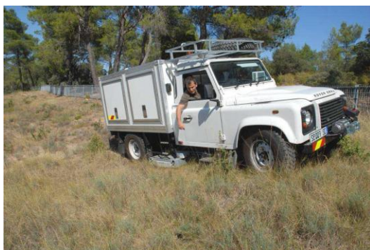
Figure 2. The VEgAS mobile laboratory. It integrates several gamma spectrometers : a NaI spectrometer (crystal volume 2.4 L, efficiency 30%), and two DSP10 ( ^{134-137}\text{Cs} detection limits are 70, 100 and 200 Bq \text{mg.kg}^{-1} , depending on vehicle speed, 2.6 km, 5 km and 10 km/h, respectively).
