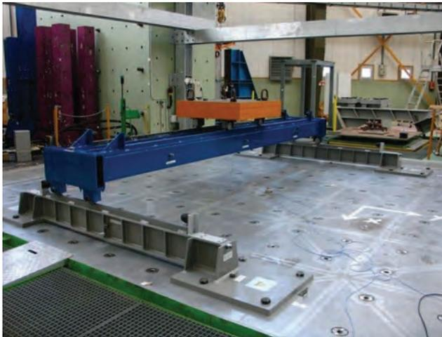
**Figure 7.10.** Handling crane undergoing testing on the AZALÉE shaking table at the CEA Saclay research centre. © CEA.
